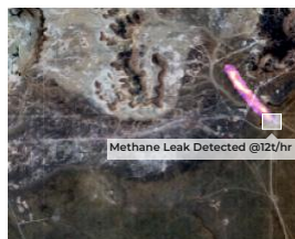
Hyperspectral for GHG Emission Detection & Quantification (ESA)
